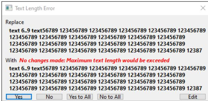
When a change would cause the text to exceed 255 characters then the macro will not be able to make that change and instead will display a confirmation dialog such as that shown at left. If you wish to manually change the text then you can press the [Edit] button at the bottom right of the dialog - this will enable you to manually make changes to the text (which you then need to confirm by pressing the [Yes] button). Manual changes can not exceed the 255 character limit.
